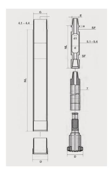
The *Lumetrix* makes it possible to create a cased borehole. The casing is used for safe installation in unstable soils of anchors or piles.
